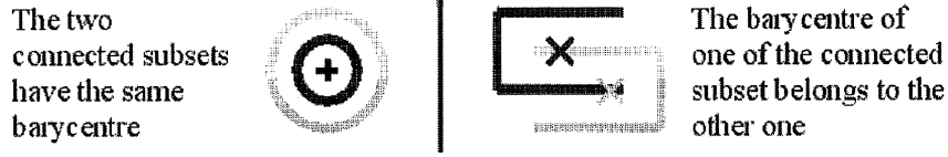
Figure 3. Weakness of barycentre concept with connectivity notion
